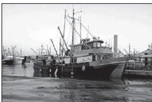
P2000M – 58 X 16 TOPHOUSE FROSTAD, 8V71 GMC MAIN, TWIN DISC GEAR, 3 STATION HYD STEERING, 3500 GAL FUEL, 700 WATER. PACKS 80K IN SLUSH IN 3 INSULATED, GLASSED HOLDS. BOOM W/TOPPING AND VANGING. ELECTRONICS INCLUDE FURUNO RADAR, RAYTHEON SOUNDER, ECHOTEC PLOTTER, FURUNO GPS, WAGNER MK IV PILOT. CURRENTLY SET UP FOR LONGLINE. EASY CONVERSION TO JUST ABOUT ANYTHING ELSE. BIG GALLEY. STATEROOMS IN CABIN AND TOPHOUSE. JUST ADD YOUR GEAR AND GO. REDUCED TO $79K.
