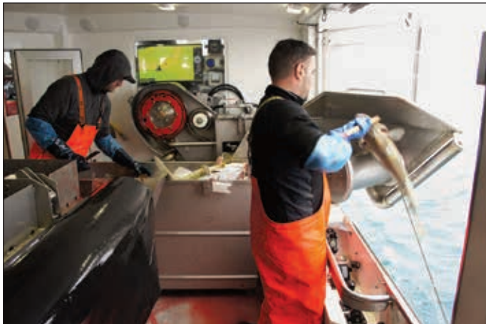
Crewmen haul cod with a Mustad Autoline Coastal System. The Coastal system is for smaller boats, while Mustad's DeepSea system is for vessels of 70 feet and longer.
