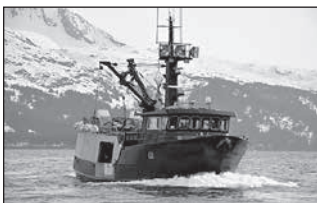
P2202M — 58 X 22 X 10.5 STEEL COMBO BUILT IN 1992, CAT 3408 MAIN, ZF GEAR, 80KW AND 30KW AUX, 18 TON AND 25 TON RSW FOR 3 HOLDS THAT PACK 125K TOTAL. LOADED WITH UP TO DATE REDUNDANT ELECTRONICS INCLUDING OLEX, SIMRAD ES70 AND FURUNO TZ TOUCH. RIGGED FOR SEINE, POT FISHING AND SET UP FOR LONGLINE WITH COMPLETELY ENCLOSED SHELTER DECK W/MARCO MKII AUTO LONG LINE SYSTEM INCLUDING 40 SKATES OF GEAR. VERSATILE LIMIT BOAT THAT CAN DO IT ALL FOR ONLY $1.725M.
