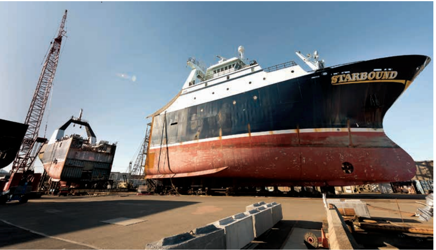
The Starbound, a Bering Sea pollock factory trawler, is being lengthened by 60 feet. Jeff Pond photos
