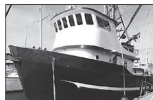
P2197M — 58 X 19.2 TOPHOUSE STEEL COMBO, 855 CUMMINS MAIN, TWIN DISC GEAR, 45KW AND 50KW ISUZU GEN SETS, 20 TON RSW W/TITANIUM CHILLER, PACK 75K IN 2 HOLDS. PACKS 4000 GAL FUEL, 800 WATER. ELECTRONICS INCLUDE FURUNO RADAR, GPS, SOUNDER, NOBLETEC, SEA SSB, ROBERTSON PILOT. WELL MAINTAINED. NICE SIZE LIMIT BOAT. GREAT SEA BOAT. $700K.
