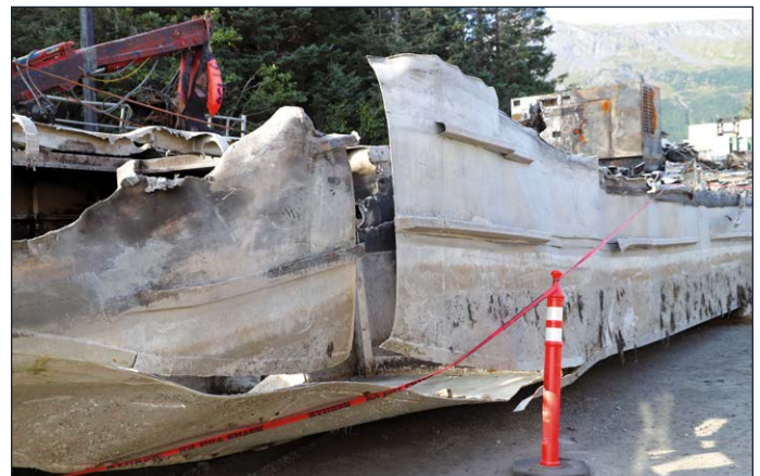
The salvaged vessel, with damaged forward side plating of port pontoon. NTSB photo
