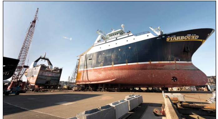
The Starbound, a Bering Sea pollock factory trawler, was lengthened by 60 feet in 2015. Jeff Pond photo
