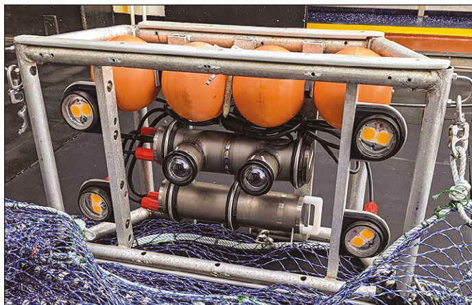
The CamTrawl net-mounted stereo camera. The middle housing contains the two cameras. The four outer cylinders are LED strobe lights that flash when the cameras fire. NOAA Fisheries photos
