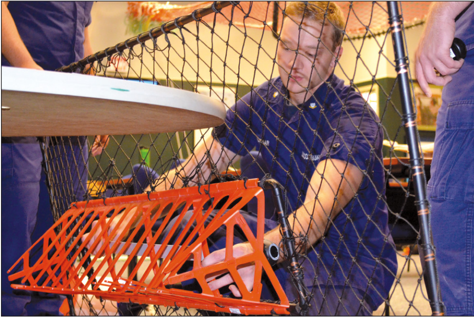
Petty Officer 3rd Class Nathaniel Cassar measures a tunnel opening on a fish pot to verify the opening meets regulations, allowing undersized or juvenile marine life to escape. Lt. Heather Bacon-Shone photo
